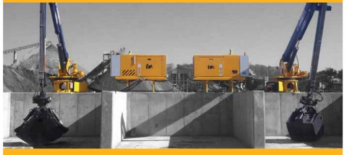
**SM-H** Power Unit: Remote | Operator Station: On loader
